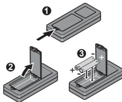
Change batteries when battery symbol is empty.
