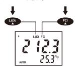
b.Temperature unit: Switch the device to °C or °F mode, and read the ambient temperature value on the LCD.
